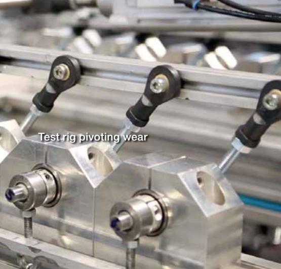
Test rig pivoting wear
