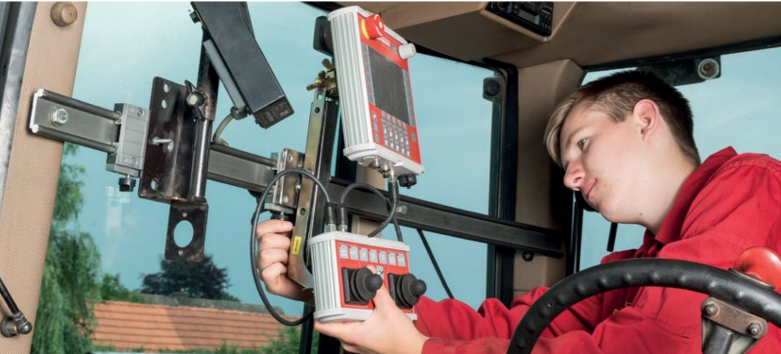
The rail allows operators to conveniently position screens and control boxes, and then simply slide them out of the way when they're not in use.
